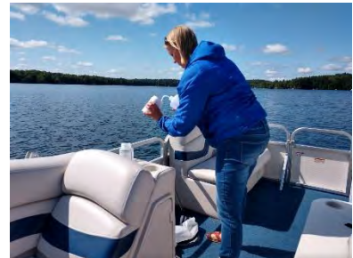
Lisa adds preservative to sample for submittal to testing lab.
